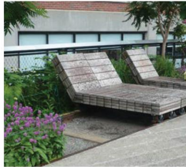
The High Line: Rail lines embedded in plaza space are activated with seats that are movable along the tracks and re-purposed to frame planting space
